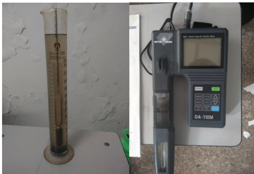
Figure 4-4. Photos of solution concentration (left) hydrometers and (right) liquid density meter
